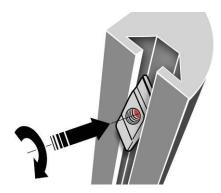
Fig. 22: Turning the sliding block
