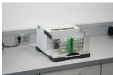
Fig. 1: Mixer Mill MM 400 with adapter for 8 conical centrifuge tubes
