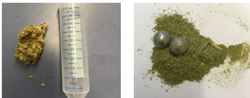
Figure 2: Flower buds before and after grinding in a 50 ml Falcon tube using the Mixer Mill MM 400
