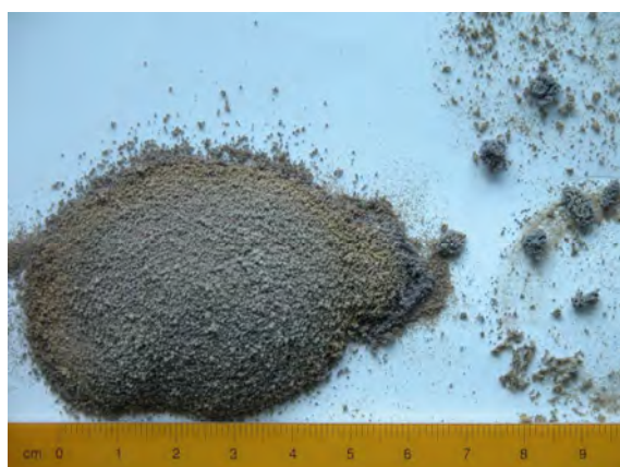
Fig. 3: sample 2 after grinding in CryoMill
