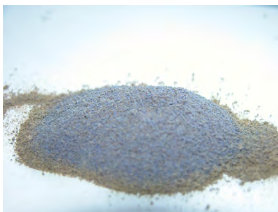
Fig. 4: sample 2 after grinding in CryoMill
