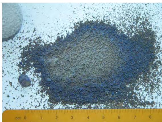
Fig. 3: sample 1 after grinding in CryoMill
