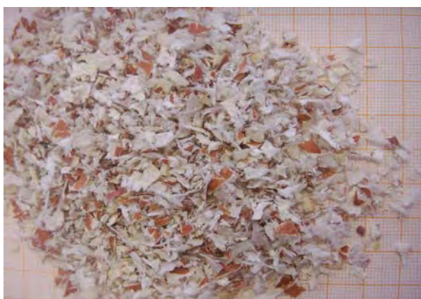
Fig. 3: After pre-grinding in SM 2000
