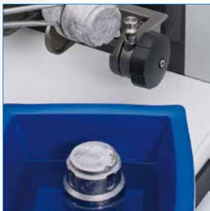
Cooling a jar in liquid nitrogen
