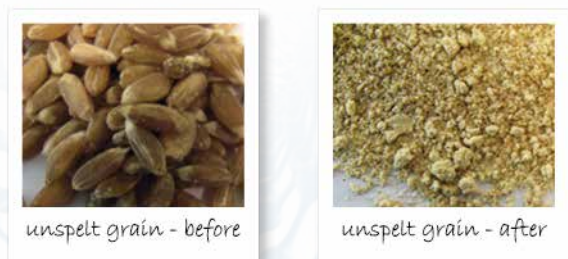
Fig. 6: Grain before and after complete homogenization in the new GM 200
