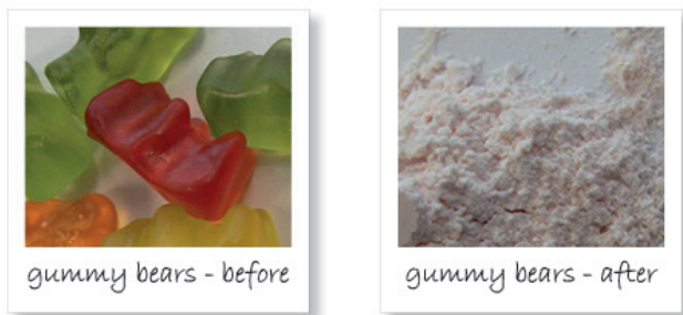
Figure 2. Gummy bears before and after cryogenic grinding in the Mixer Mill MM 400
