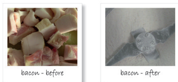
Figure 4: Bacon before and after grinding in the Knife Mill GRINDOMIX GM 300
