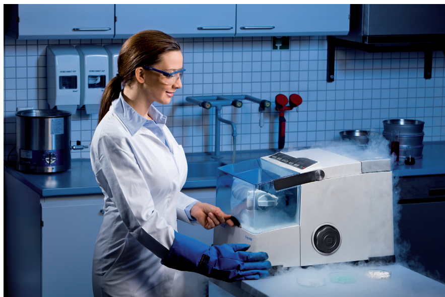
Figure 1. The CryoMill offers the advantage of continuous cooling of the grinding jar with LN 2
