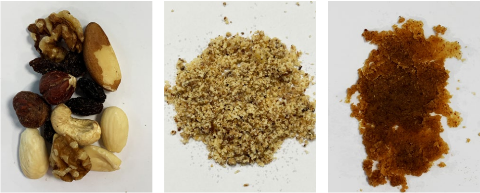
Fig. 3a: Mixed nuts: original sample (left), ground optimally (middle, GM 200) and over-ground (right, GM 200).
