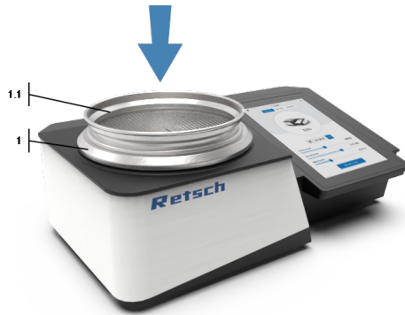
Fig. 8: Insert analysis sieves 203 and 200 mm
