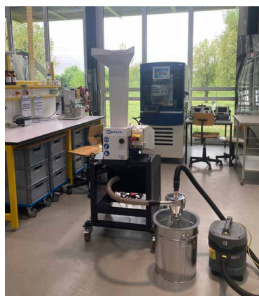
Fig. 5: left: HM 200 equipped with cyclone right: Biochar-based fertilizer granules
