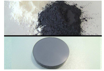
FeSiMg-Granulate 12 g plus 2 g licowax Particle size 0.10 mm Pressing tool 40 mm Aluminum cups 60 s 15/25/35 tons
