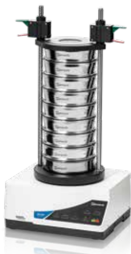
Vibratory Sieve Shaker AS 200 control
