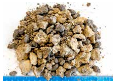
Soil/stone agglomerates pre-crushed in Jaw Crusher BB 50
