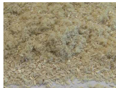
Figure 2: Pre-cut stems of hemp plants before (left) and after grinding in the Cutting Mill SM 300 (right)
