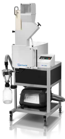
Fig. 1: Cutting Mill SM 300 with cyclone
