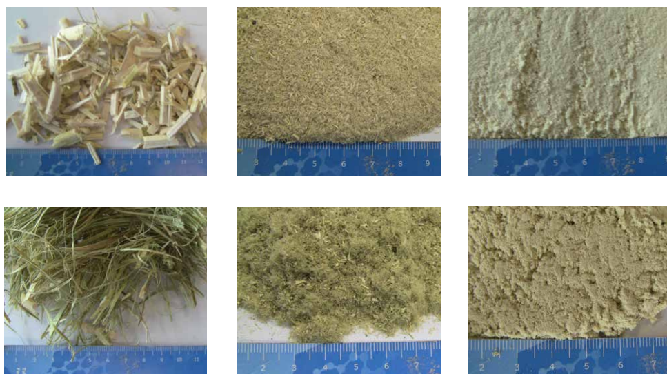
Figure 4: Hemp hurd (above) and hemp fibers (below) after pre-cutting in the SM 300 and subsequent pulverization in the SR 300.
