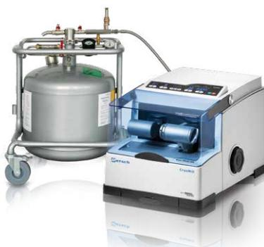
CryoMill with a 50 liter liquid nitrogen container
