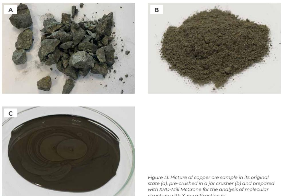
Figure 13: Picture of copper ore sample in its original state (a), pre-crushed in a jar crusher (b) and prepared with XRD-Mill McCrone for the analysis of molecular structure with X-ray diffraction (c).
