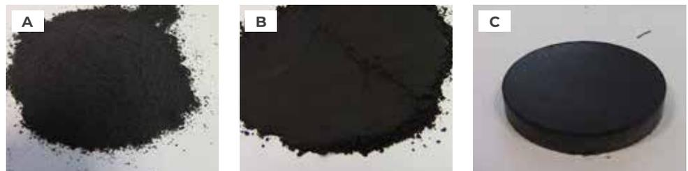
Figure 12: Sample of manganese oxide before (a) and after the milling process in the PM 100 (b). For XRF analysis the sample is pressed into a pellet (c).
