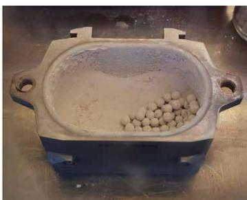
Figure 9: Sulphidic solid electrolyte (LPS) together with some balls in a 125 ml Screw-Lock jar of the MM 500 control, opened in a glove box.
