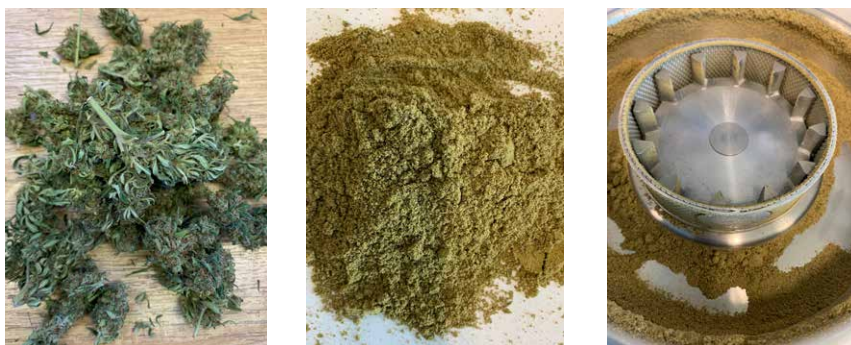
Fig. 7: Cannabis flowers before and after cryogenic grinding in a ball mill (a total of 4 min for 20 g sample) or the ZM 300 (10 min for 500 g sample).
