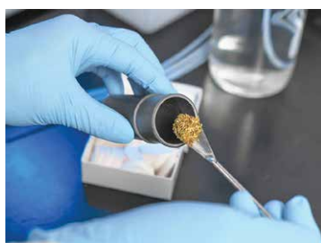
Fig. 2 - above: Extraction system EDGE below: pouring the homogenized sample into the Q Cup before extraction
