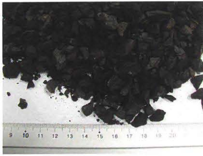
Figure 4. Lignite sample after pre-crushing in the BB 500 XL with 6 mm gap width setting
