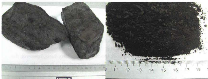
Figures 2 and 3. Lignite before (left) and after crushing in the BB 500 XL (right). With a gap width setting close to zero, the greater part of the sample showed a particle size below 1 mm.
