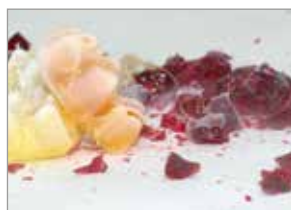
Material embrittled with liquid nitrogen
