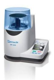
The cutting effect generated by the sharp steel blades of the knife allows for very effective size reduction of samples with a high water, oil, sugar or fat content. The GM 200 covers a wide application range from grainy food stuff such as rape seed, rice, soy beans or corn to fibrous or tough samples such as meat, fish, sticky candy or cheese. The mill features three different operation modes (standard mode = cutting, reverse mode = impact, interval mode =
