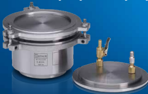
Grinding jar "comfort" for PM series with safety closure, aeration cover
