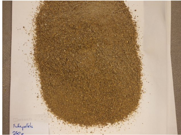
Picture 2: Feed pellets after grinding with a 3 mm sieve
